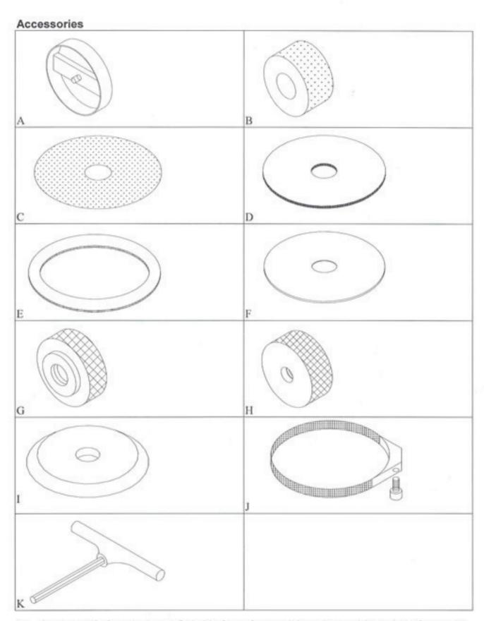
A . Cutting knife for specimen: Suitable for soft material, such as rubber, cloth, foam, etc.
